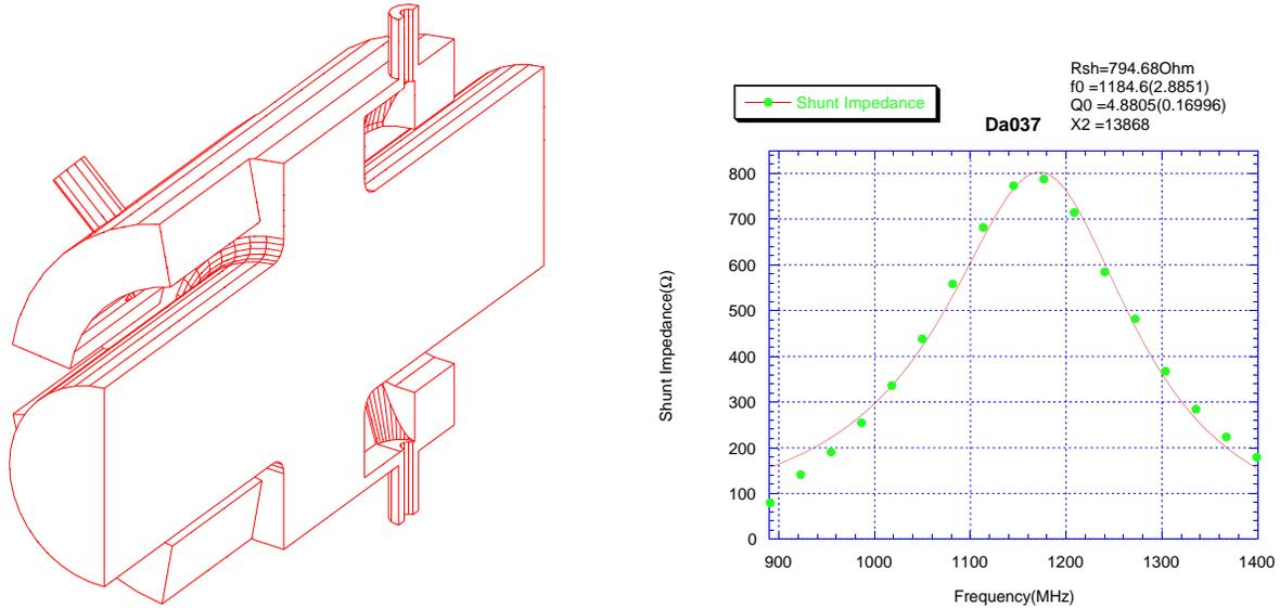
**FIGURE 7.** HFSS model of the wageguide overloaded cavity as the longitudinal kicker and the calculated shunt impedance. The value includes the transit time factor.
