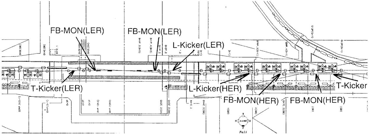
**FIGURE 6.** Arrangements of the feedback components in the Fuji experimental hall.
