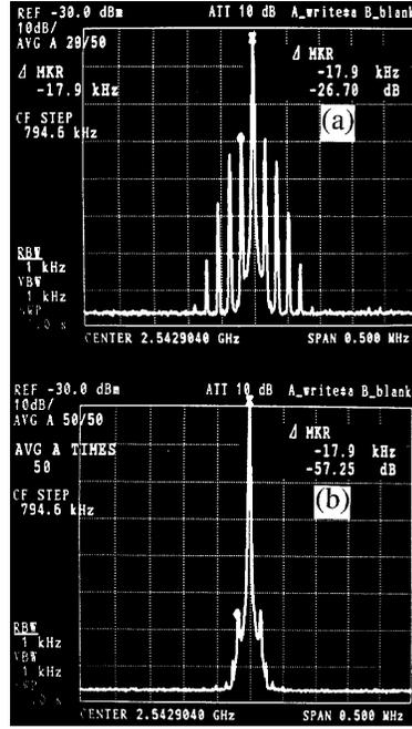
**FIGURE 5.** Beam spectra, (a) with longitudinal feedback off (b) with longitudinal feedback on. Without the feedback, there appeared many synchrotron sidebands corresponding to the strong longitudinal oscillations. The amplitude of the first sideband has reduced down to -30dB with the longitudinal feedback on. The total beam current was about 120 mA.
