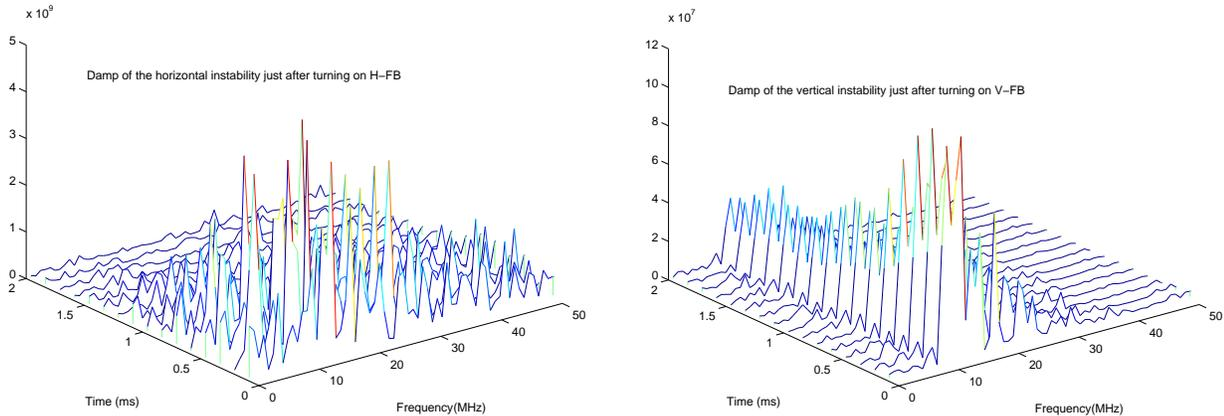
**FIGURE 4.** Damp of the horizontal and vertical coupled bunch oscillation observed with the two-tap FIR filter.
