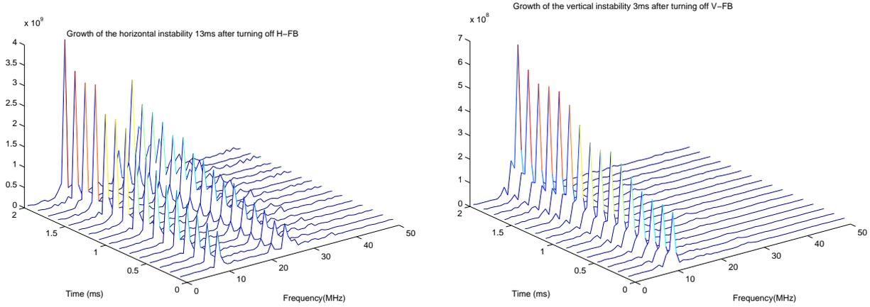
**FIGURE 3.** Growth of the horizontal and vertical coupled bunch oscillation recorded in the two-tap FIR filter.
