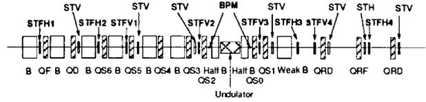
Figure 4: Arrangement of the orbit feedback system
