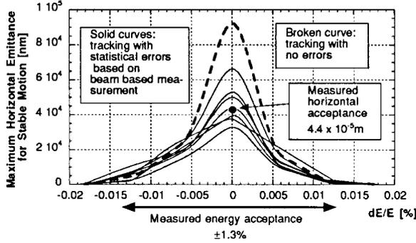
Figure 2: Comparison of acceptance between the measurement and the simulation
