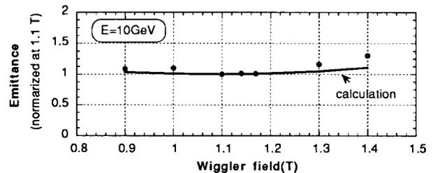
Figure 1: Emittance vs. field of the damping wigglers
