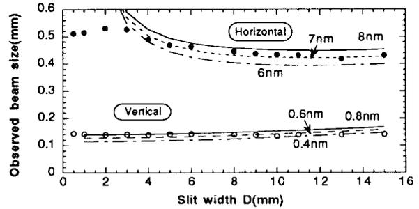
Figure 7: Observed beam size vs. the slit width
