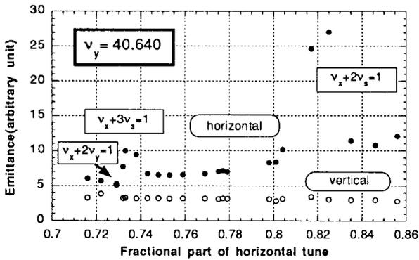
Figure 3: Horizontal tune vs. emittance
