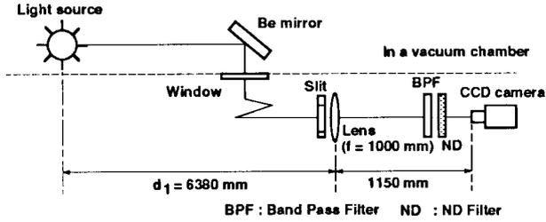
Figure 6: Experimental setup of the emittance measurement
