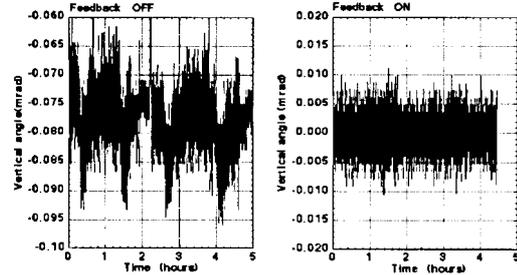
Figure 5: Change of vertical angle at the source point with and without the orbit feedback
