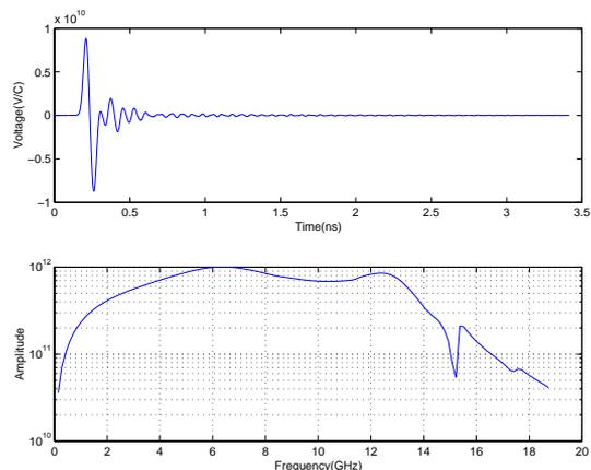
Figure 2: Simulated output of a BPM for 4 mm bunch using MAFIA T3 (upper) and its Fourier transform (lower).
