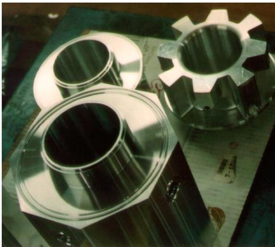
Figure 5: Photo of the DAΦNE type cavity under fabrication.
