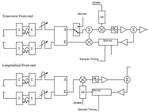
Figure 3: Block diagram of the front-end circuit of the transverse and the longitudinal detection system.
