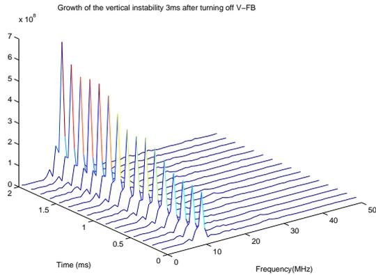
Figure 4: Growth of the vertical coupled bunch oscillation recorded in the two-tap FIR filter.
