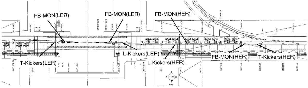
Figure 1: Location of the feedback instruments at Fuji crossing area. Positrons comes from left side and electrons comes from the right side. The local control room for the feedback system is located under the accelerator tunnel (B4 level). Feedback amplifiers will be installed under the crossing bridge.
